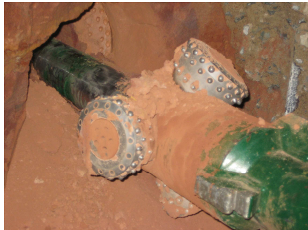
Low-torque rock reamer
