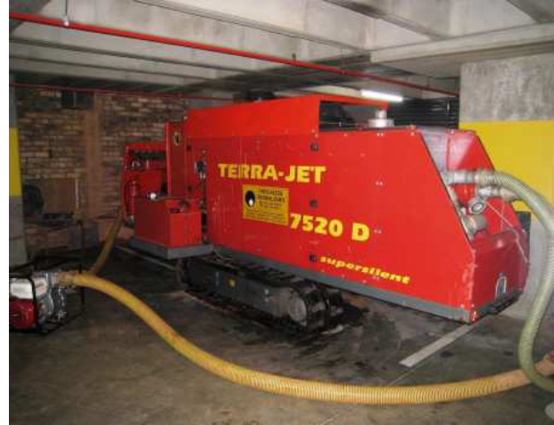
The remodelled TJ 7520 drill - all of 1,8 m high
