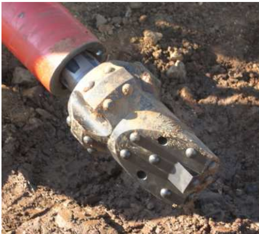
Air percussion head, diameter 95 mm
